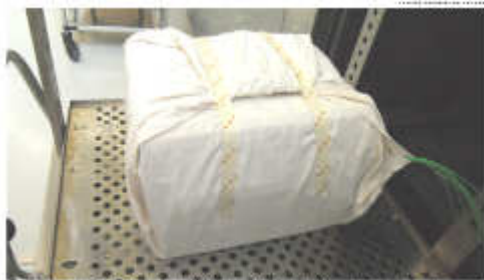
Fig. 2. Schematic diagram of the test load in the chamber of the sterilizer. A schematic diagram of the test load in the chamber of the sterilizer.
