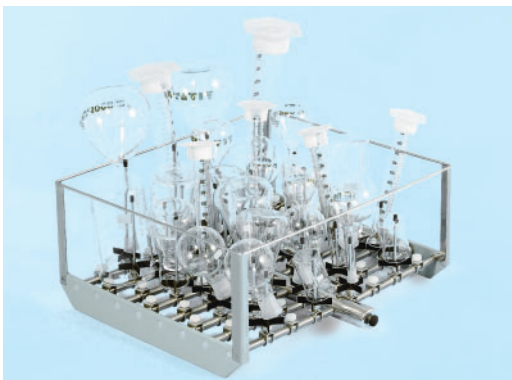
Multi-nozzle rack, art. no. 820 362 For intensive cleaning of diverse laboratory utensils such as volumetric flasks, measuring cylinders etc. Multi-nozzle rack with 32 nozzles (up to 56 nozzles possible), fitted with: 4 nozzles \varnothing 6 mm x 200 mm, 6 nozzles \varnothing 6 mm x 150 mm, 6 nozzles \varnothing 5 mm x 150 mm and 16 nozzles \varnothing 5 mm x 110 mm.
